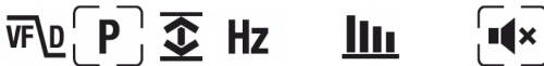
Figure 5.2 Mode icons (AC voltage measurements): Peak mode and Silent mode are enabled
