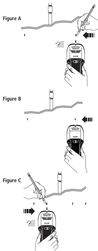
4. **(Figure C)** To continue to reduce sensitivity and further refine the scanning area, repeat Step 3. This procedure can be repeated multiple times to narrow the field even further.
