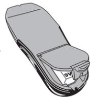
**Low Battery Indicator:** The Low Battery Indicator icon displays when the battery level is getting low. While the tool will still operate, the battery will need to be replaced soon. When the battery icon begins to flash and is the only icon displayed on the screen, the battery level is too low and not sufficient to power the tool for proper operation. Please replace the 9V battery with a brand new battery immediately.
