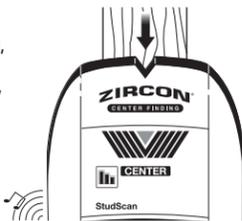
In cases of deeper studs (thicker walls), when the centre of the stud is located only two bars will show on the Signal Strength Indicator and only the SpotLite® Pointer and middle segments of the Target Indication bars will illuminate. If you still cannot locate a stud, try DeepScan® mode.
