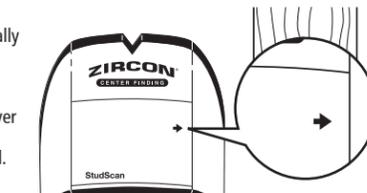
**ACT™ (Auto Correcting Technology):** During scanning, the tool will automatically recalibrate itself when needed. This recalibration is transparent and no indication is made. If an arrow icon illuminates, the tool calibrated near or over a stud and then moved away. The arrow indicates the direction of the missed stud.
