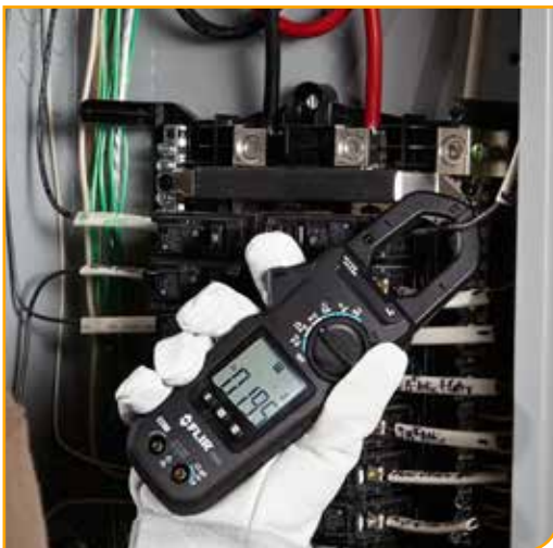
Accu-Tip levert exactere stroommetingen
